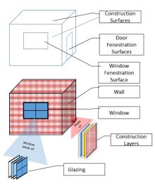
Figure 3: Logical representation of the building created from the 2D sketcher, which includes building geometry, orientations and surfaces. This enables the user to test various materials against these building construction components.
