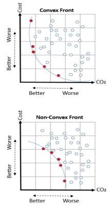
Figure 6: Illustrates the two typical types of Pareto fronts: convex and non-convex.
