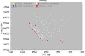
Figure 7: Results obtained from simulating a basic box model. The red points represent a convex Pareto front (Adapted from Huws and Jankovic, 2014).
